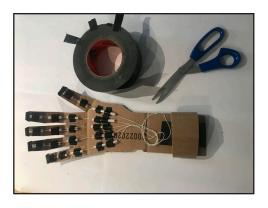
5. Add an Arm Brace: Loop a one inch wide length of cardboard around your palm, not including the thumb. Trim any extra cardboard so there's no overlap. Tape this loop to your cardboard arm.
